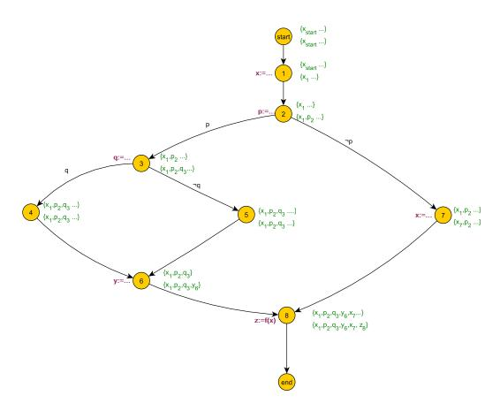
Figure 2.4. CFG Showing Reaching Definitions.
