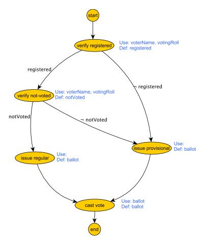
**Figure 3.12.** CFG Annotated With Data Flow Information Of "Issue ballot and get vote" System.
