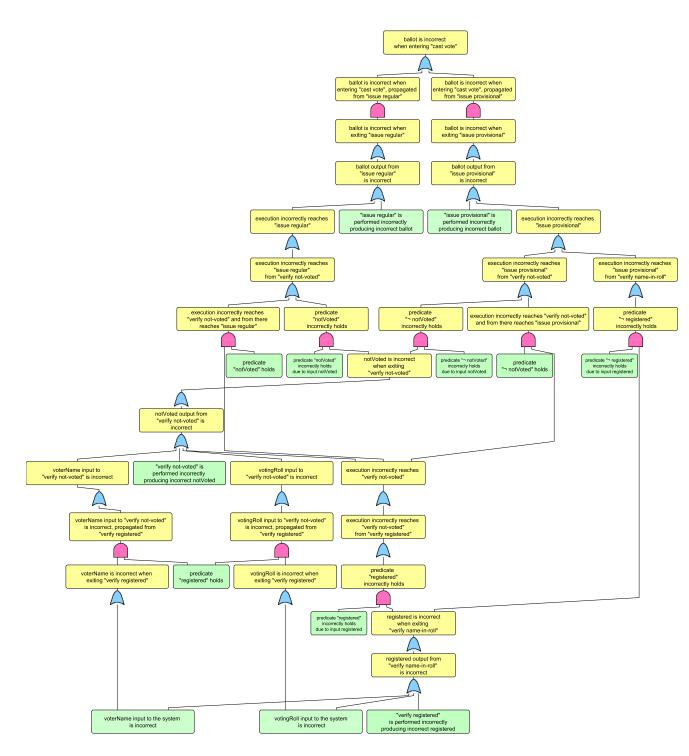
**Figure 3.14.** Initial FT Derived From "Issue ballot and get vote" System Model Given The Top Event "ballot is incorrect entering 'cast vote'".
