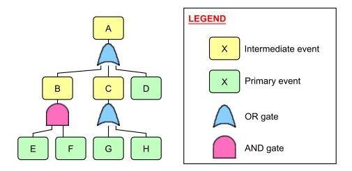
Figure 2.1. Fault Tree Example.
