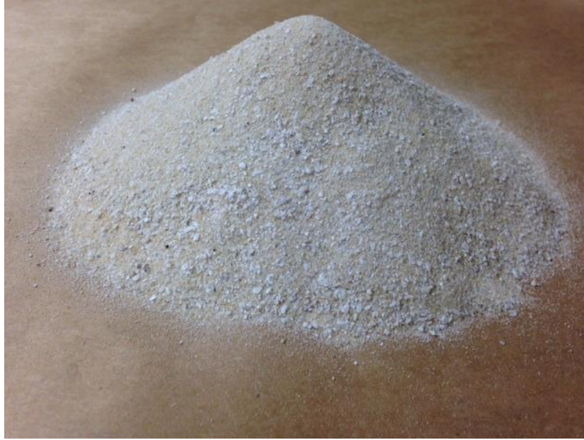
Figure 4.1 Soil M30 (sand with 30 % gypsum)
