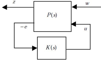
Figure (3.2): Standard LFT diagram for  $H_\infty$  optimal control design
