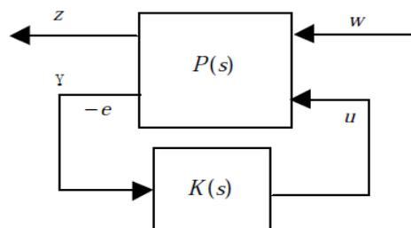
Figure (2.13): Standard LFT diagram for  $H_2$ -optimal control design
