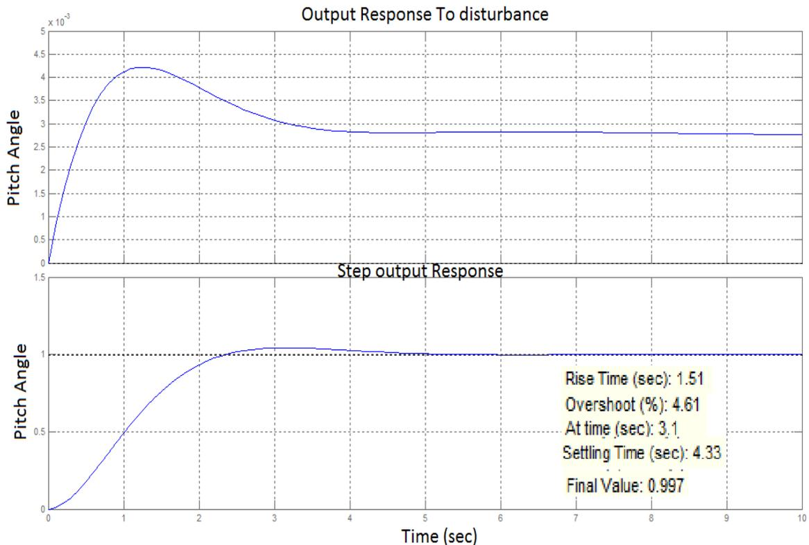
**Figure (4.9): Step response close-loop system and output disturbance**
