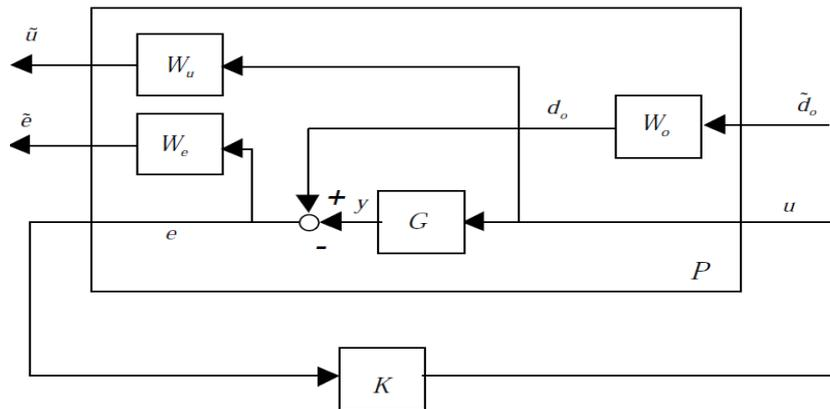
Figure (2.18): Typical setup for  $H_\infty$ -optimal control design
