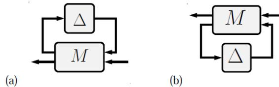
Figure (1.2): LFT (a) upper LFT  $\Delta * M$ . (b) lower LFT  $M * \Delta$ .
