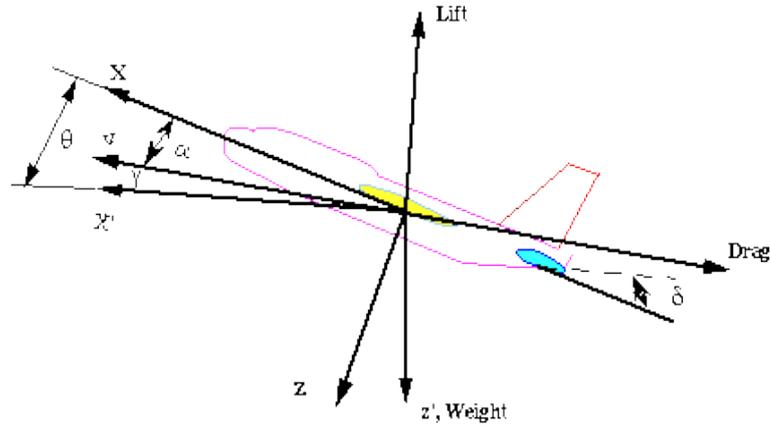
Figure (4.2): The basic coordinate axes and forces acting on an aircraft [59]
