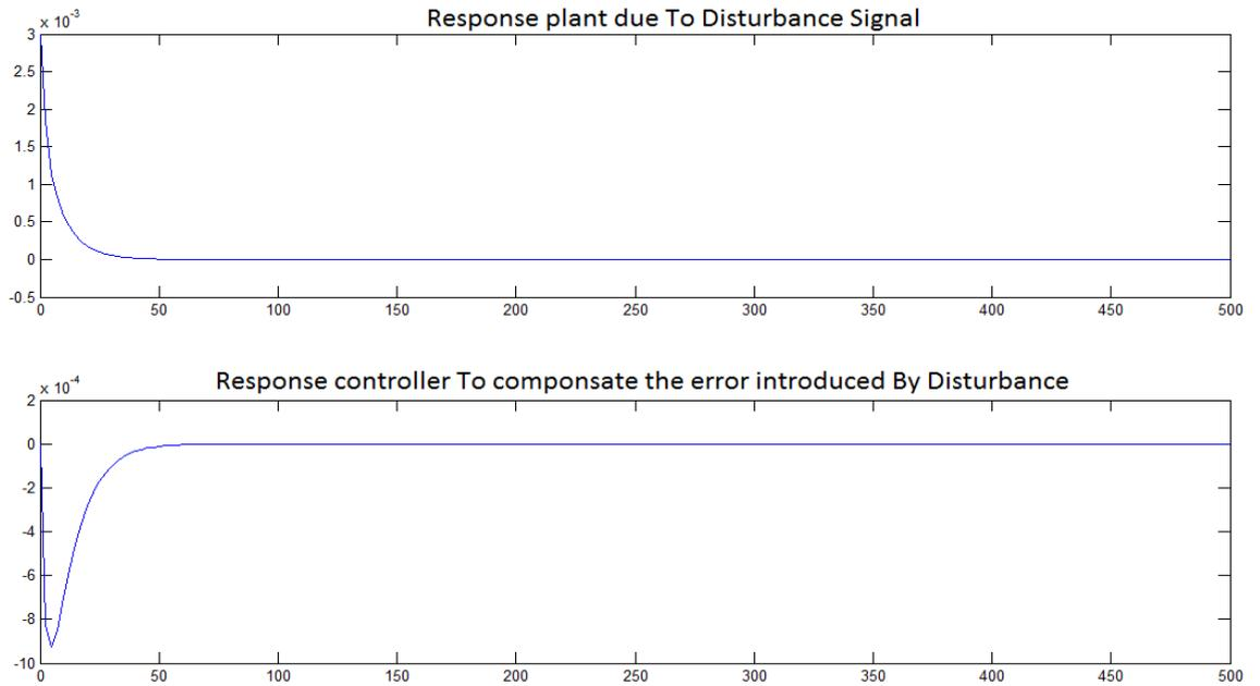
**Figure (4.13): Plant and controller response due to introduced disturbance input**
