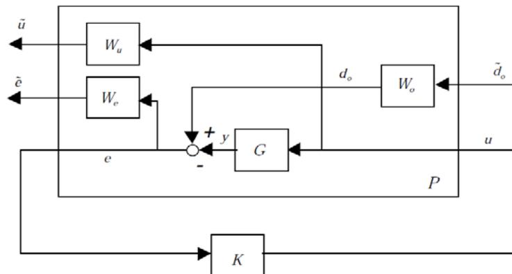
Figure (2.12): Typical setup for  $H_2$ -optimal control
