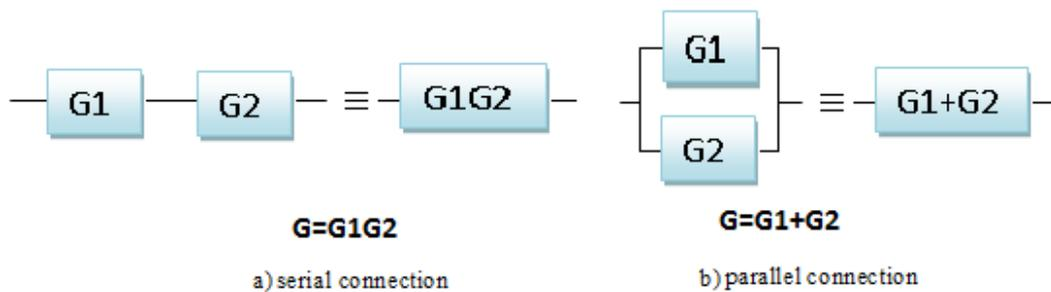
Figure (1.3): connections a) serial connection b) parallel connection
