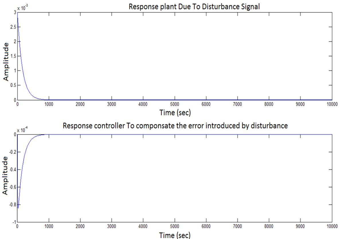
**Figure (4.8): Plant and controller response due to introduced disturbance input**
