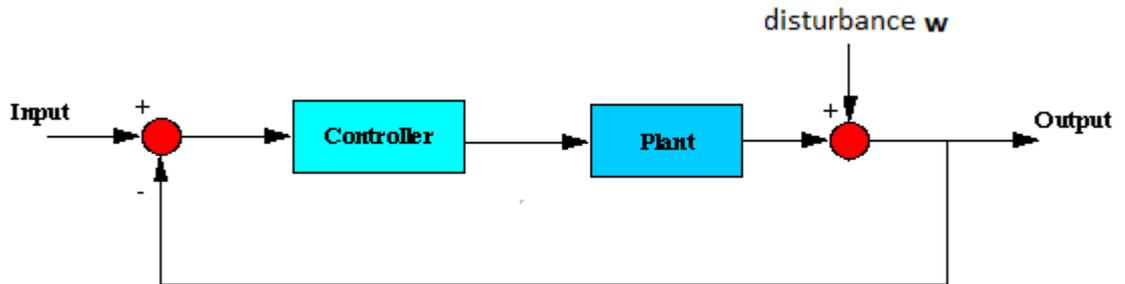
Figure (4.7): Close-loop feedback with controller and plant
