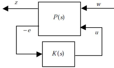
Figure (3.1): Standard LFT diagram for  $H_2$  optimal control design
