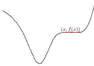
Figure (2.21): A Quasiconvex function  $f$  on  $\mathbf{R}$ , with a locally optimal point  $x$
