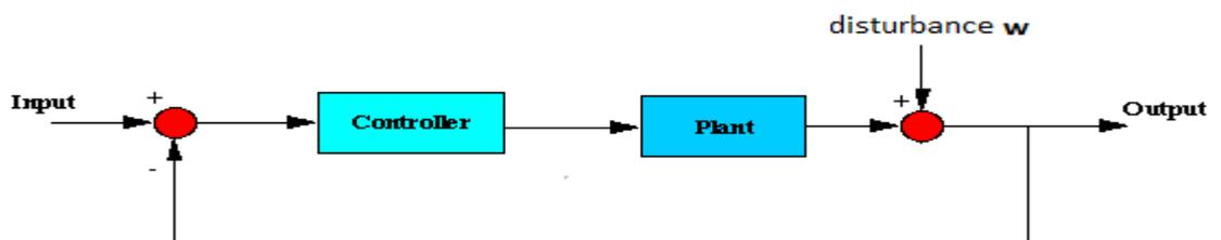
Figure (4.12): Close-loop feedback with controller and plant
