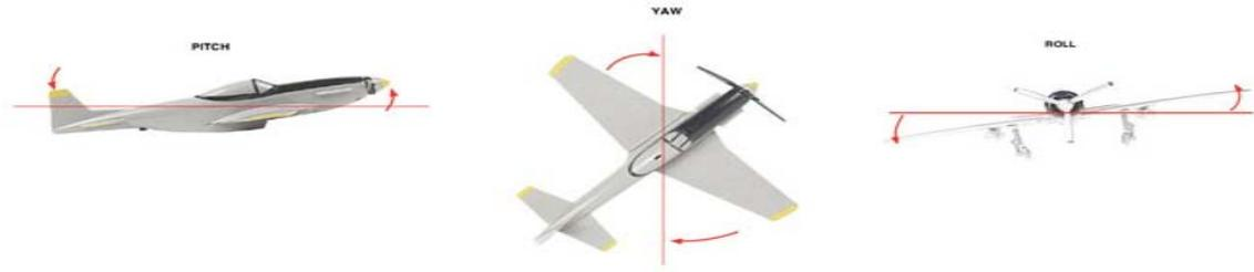
Figure (4.1): Pitch-yaw-roll coordinate axes of aircraft [59]
