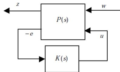
Figure (2.19): Standard LFT diagram for  $H_\infty$ -optimal control design
