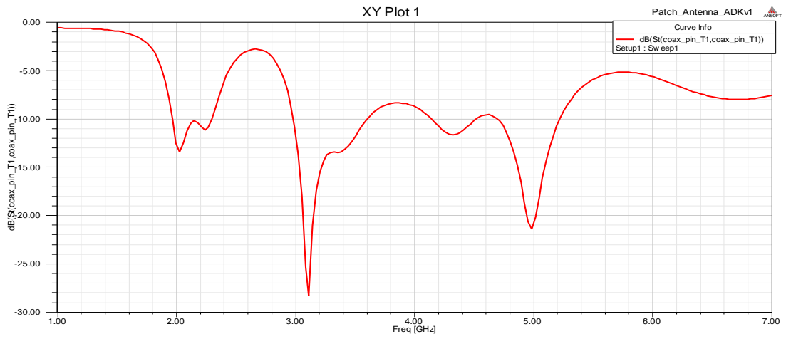
Figure 3. 13: Return loss of MSP antenna with IPF position = y cm.
