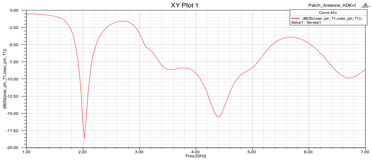
Figure 3. 21: Return loss of MSP antenna with IPF position = 3y cm.
