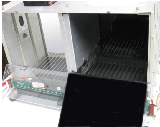
Figure 2. Photograph of the Shuttle Box. All subjects were exposed to a metal shuttle box with both light (left) and dark (right) compartments separated by a metal door.
