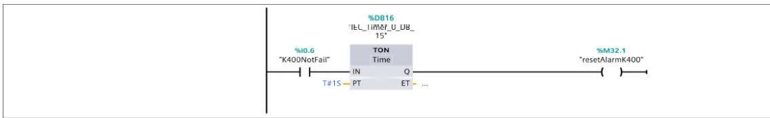
Network 40: Automatic Reset Alarm K400
