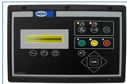
Figure (3.7) : FG Wilson generator control Panel
