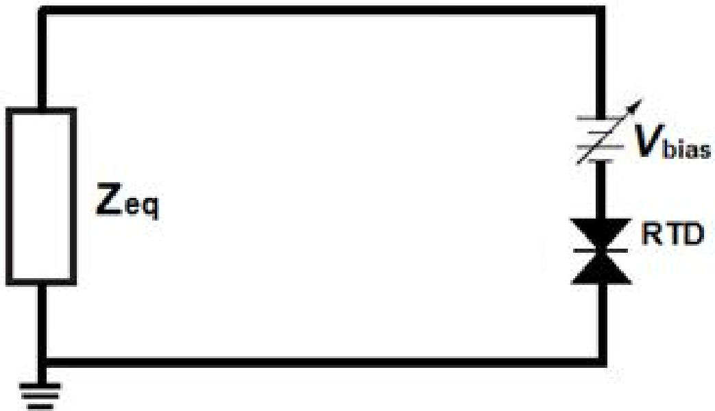
Figure 7.18: Simplified equivalent circuit model of the three cases model in figure 7.14.
