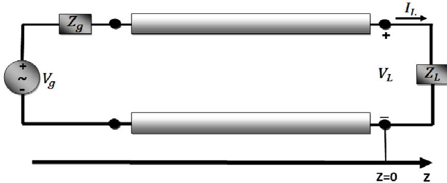
Figure 2.5: A transmission line terminated in a load impedance  $Z_L$ .
