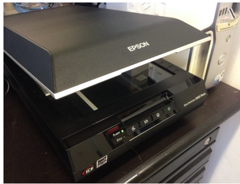
Figure 5.7 A flatbed photo scanner V800 (Epson). The calcium samples are mounted in a sample frame, and images were scanned while the sample is facing down (toward the image sensor).
