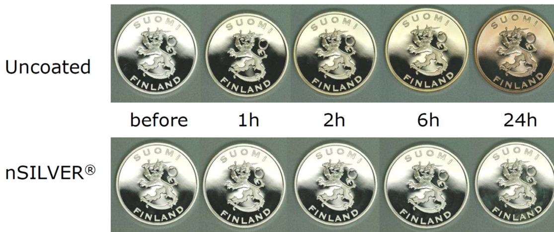
Figure 3.1 Accelerated thioacetamide tarnishing test of ALD coatings on silver coins (ISO 4538). The color of the coin without an ALD coating changes over time due to the thioacetamide exposure. Adapted from reference [139] .
