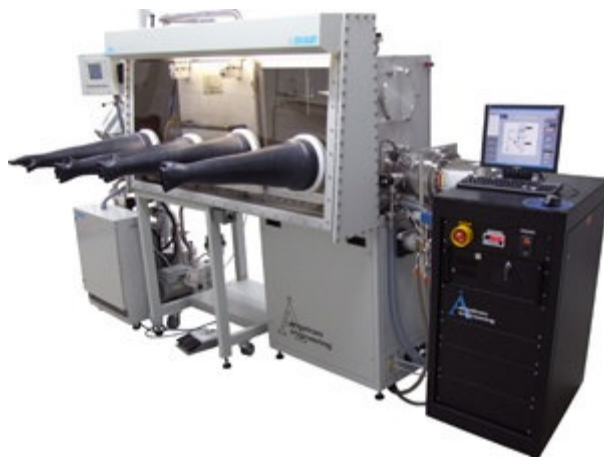
Figure 5.3 Thermal evaporation system (EvoVac, Angstrom Engineering) used for calcium deposition, which is installed in a glove box (MBraun).
