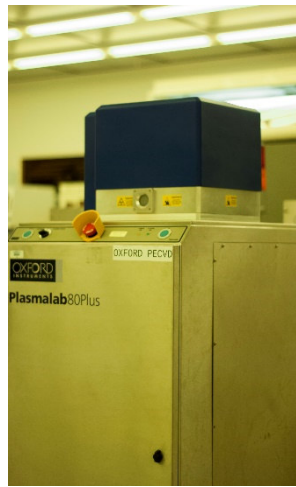
Figure 5.15 Oxford PECVD system used to deposit SiN x films at a low temperature, 100°C.
