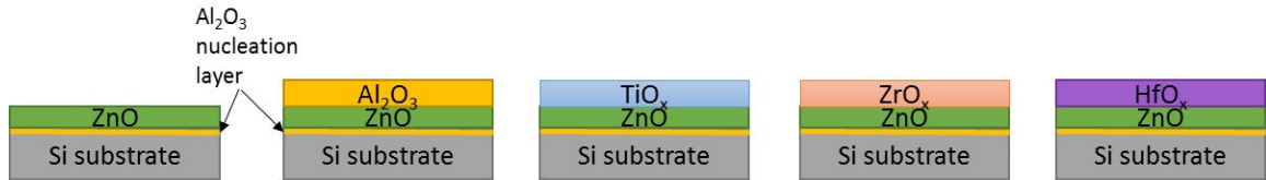
Figure 3.4 Schematic diagrams of tested ALD films in this PL study. From the left, an uncapped ZnO sensor sample, an \text{Al}_2\text{O}_3 -coated ZnO sample, a \text{TiO}_x coated sample, a \text{ZrO}_x -coated sample, and a \text{HfO}_x coated sample.
