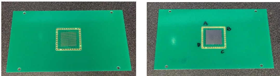
Figure 10-1 Left: daisy chain patterns on the organic board to be assembled; right: drop test sample with the four daisy chains measuring the resistance at the four corners which are the most critical locations (each corner includes 4 \times 4 compliant interconnects)
