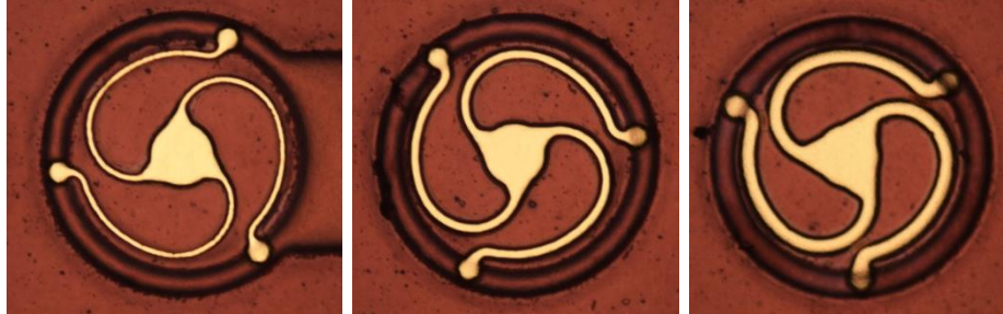
Figure 5-12 Images of plated 3-Arc-Fan compliant interconnects (from left to right: 10\mu\text{m} , 15\mu\text{m} and 20\mu\text{m} arcuate beam width)
