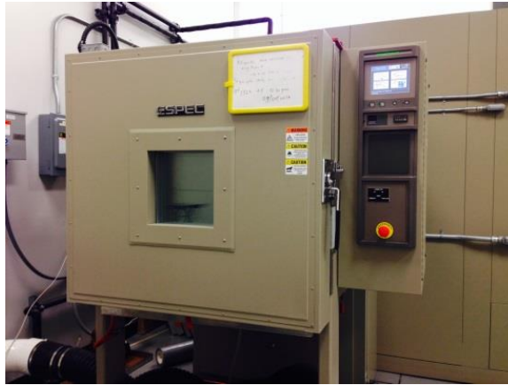
Figure 7-4 Thermal cycle chamber manufactured by ESPEC®
