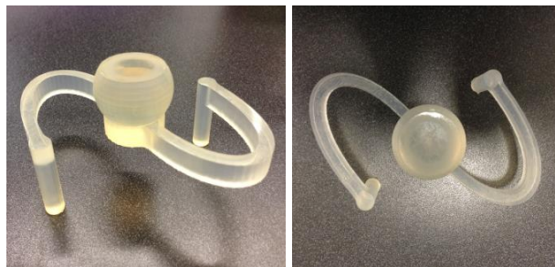
Figure 3-1 Scaled-up polymer version of the 2-Arc Fan Interconnect with second-order splines: 3-D rendering (left) and top view (right)
