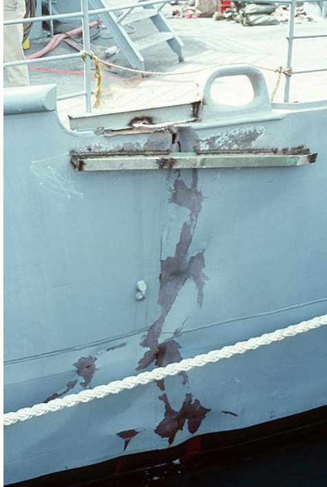
Figure 6 Cracked hull of USS Princeton. Photographs from US Navy archives.
