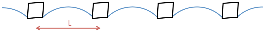
(a) Dislocation bowing against a regular linear array of SIA loops.
