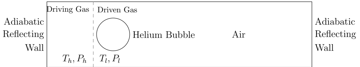
Figure 17: A simplified schematic of the Richtmyer-Meshkov instability problem in a shock tube with a helium bubble surrounded by air. The diaphragm is broken (removed) instantaneously at the simulation start time.
