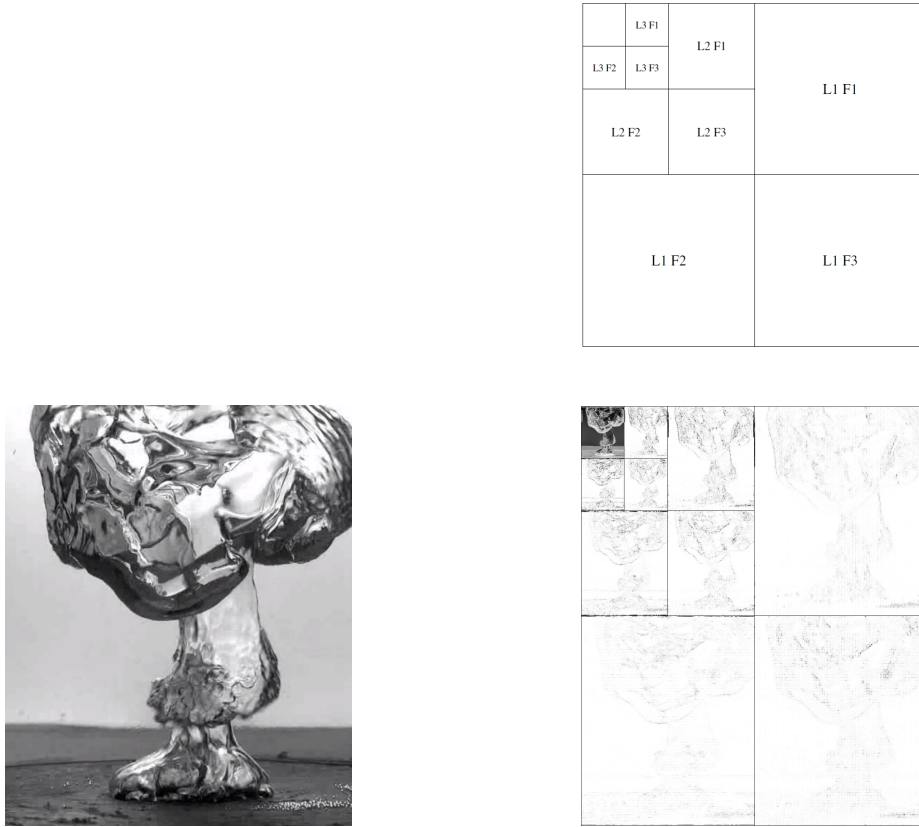
Figure 10: Multi-level wavelet representation of a 2D image from a nucleate boiling experiment with a small heater placed in the middle of a water tank [Boziuk and Glezer (2013) [14]]. The lower-left image shows the original nucleate boiling image with a vapor plume rising due to buoyancy effects. The lower-right image shows the results of multi-level wavelet decomposition. The upper-right shows a schematic of the separation of points by 2D wavelet family in the multi-level wavelet decomposition. The number preceded by ‘L’ indicates the level and the number preceded by ‘F’ is the wavelet family.
