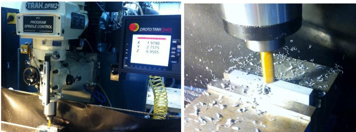
Figure 3.9: Milling of the parts for the ionic wind generator requiring a higher accuracy.
