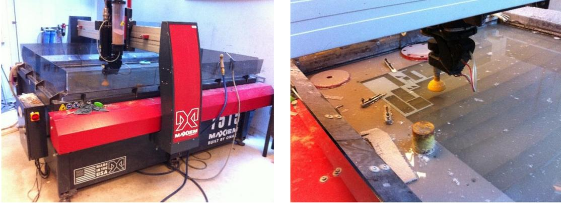
Figure 3.8: Water jet cutting of the structural part for the ionic wind generator.
