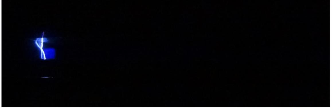
Figure 3.3: Breakdown stage for a 100 $\mu$ m wire at a voltage of 18kV.
