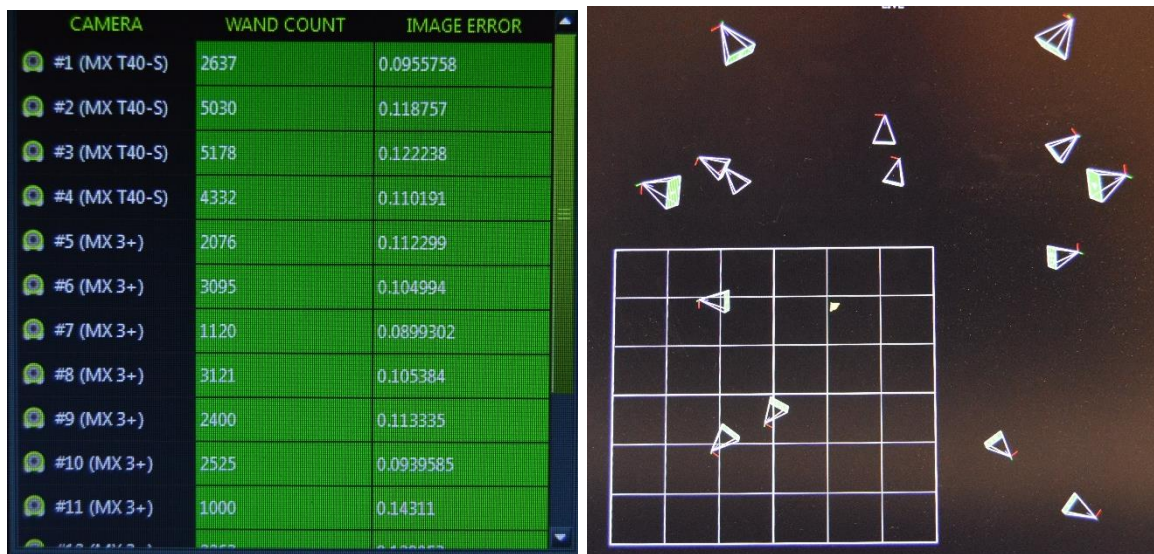
Figure 2.4: Left -- Vicon Camera Calibration Error (mm), Right -- Vicon Camera Setup
