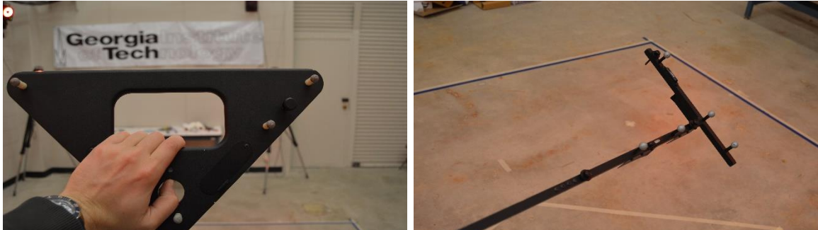
Figure 2.5: Left -- Origin Triangle to set Origin, Right – “Wand” used for Vicon Calibration
