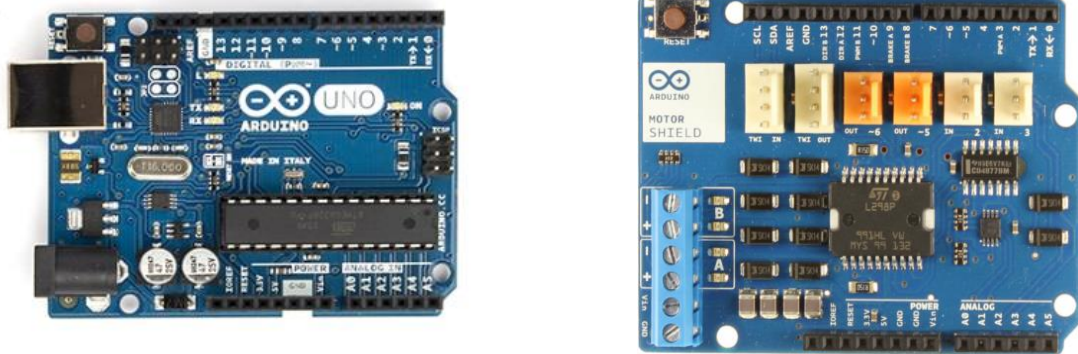
Figure 2.6: Left -- Arduino UNO Board, Right -- Arduino Motor Shield
