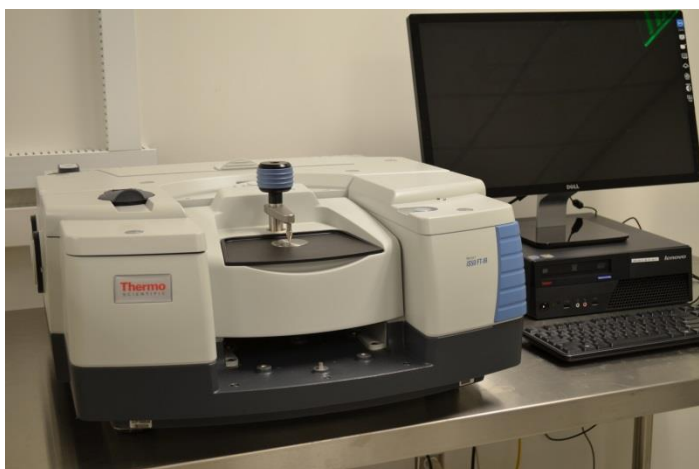
Figure 73: Thermo Scientific Nicolet iS50 FT-IR spectrometer at the Georgia Tech's Organic Cleanroom.
