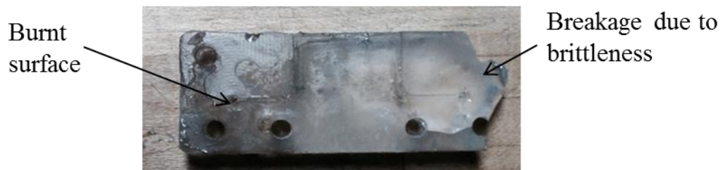
Figure 5.16: Parts post-cured at 120°C experienced pyrolysis and became extremely brittle, often breaking during the mold release.
