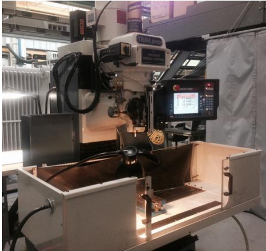
Figure 3.4: The Prototrak 3-Axis CNC mill utilized a 150,000 RPM spindle that allowed for the use of micro endmills.
