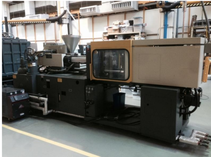
Figure 1.5: The process chain for injection molded parts converts plastic pellets to final parts in one step. Image on bottom is the Sumitomo SH75 injection molding machine in the Manufacturing Research Center at Georgia Tech.
