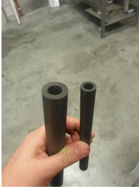
Fig. 37: Graphite pipes used in experimental loops. Pipe on the right had OD: 0.5" and ID: 0.3125". Pipe on the left had OD: 0.875" and ID: 0.5"
