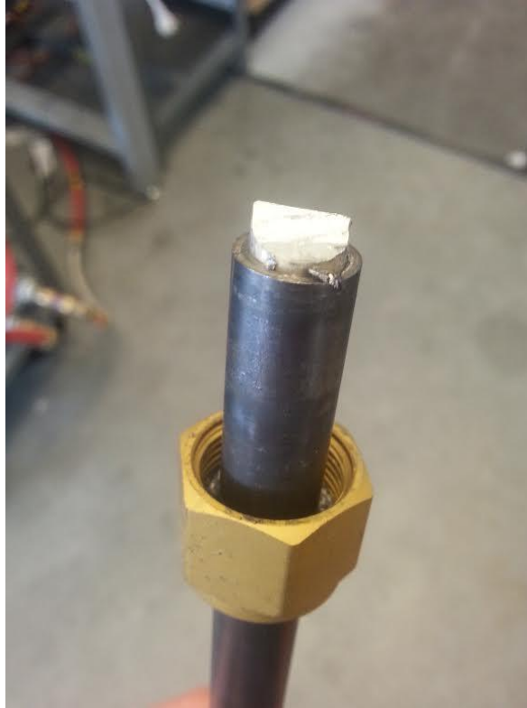
Fig. 39: Sn filled section of glass-lined stainless steel tubing
