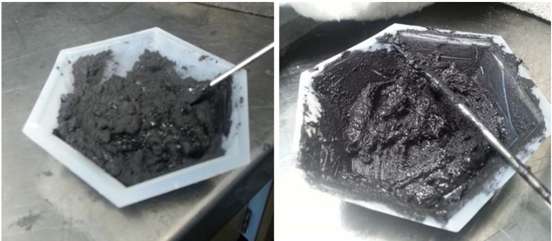
Fig. 43: Cotronics 931 cement. Left picture is unmixed, right picture is thoroughly mixed.
