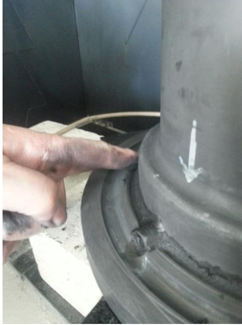
Fig. 45: Graphite 2 component cement bond. Excess cement squeezed from joint is smoothed into a beveled surface
