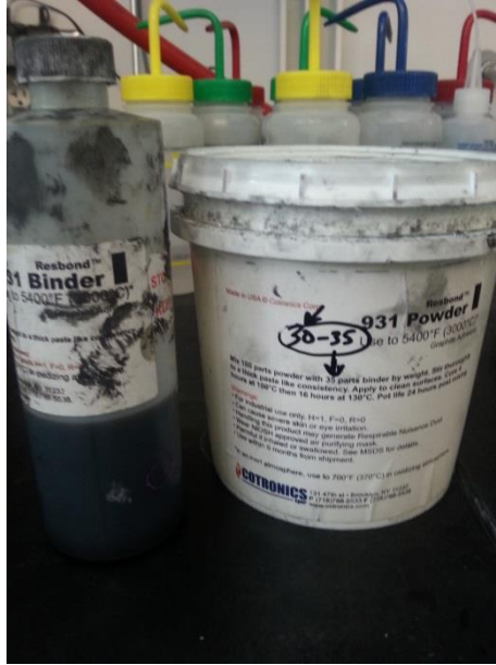
Fig. 42: Cotronics 931 graphite cement. 2 component mixture consisted of binder and powder.
