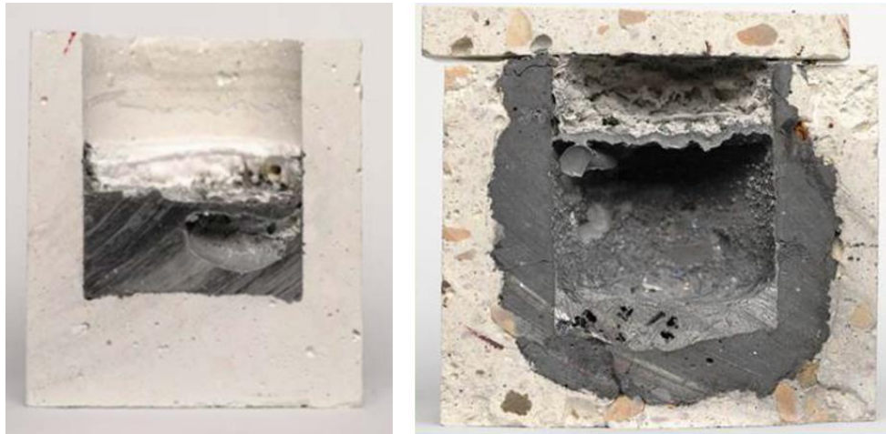
Fig. 21: Castable cement cup cross sections exposed to Al(l) at 1200°C for 120 hours. Left is WAM ALII, right is standard castable cement, WAM 45 SC. The ALII with <0.4% silica experienced no degradation. The 45 SC with 48% silica was penetrated. [75]
