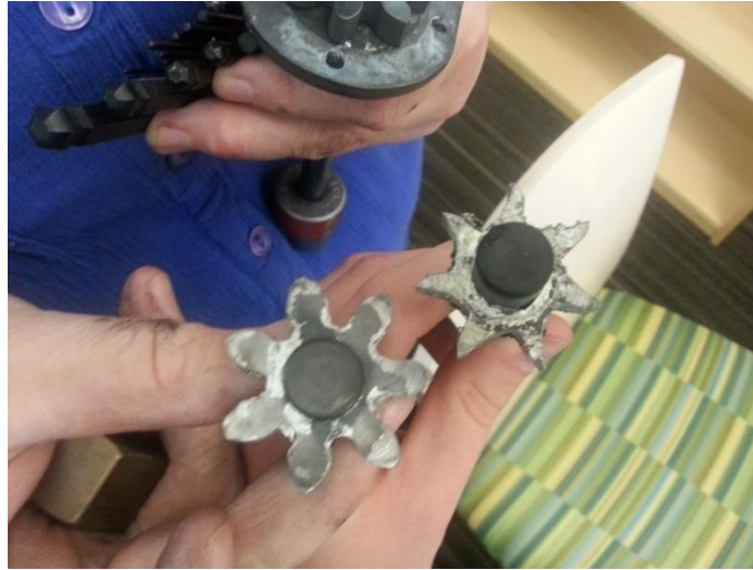
Fig. 36: Two originally identical stainless steel gears. The right gear was corroded by Sn(l) after < 24 hrs. of operation. One steel gear was treated with a ceramic coating, while the other was not, which led to a major difference in corrosion.
