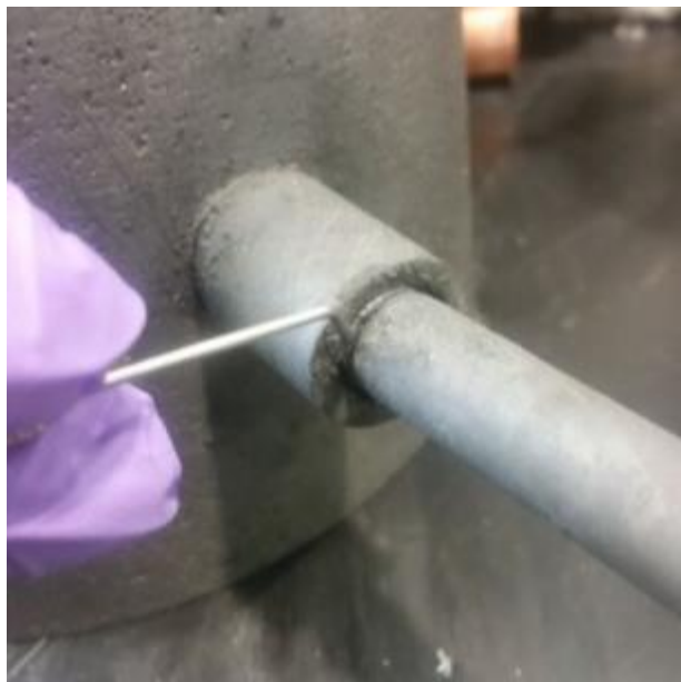
Fig. 48: Pick and cement procedure for leaking part.
