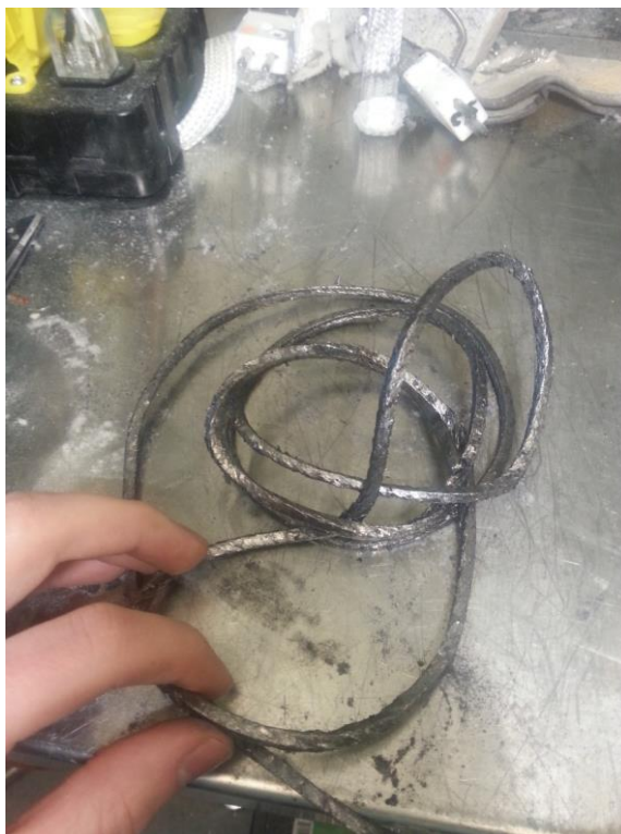
Fig. 54: Graphite rope packing that replaced PTFE and teflon seals
