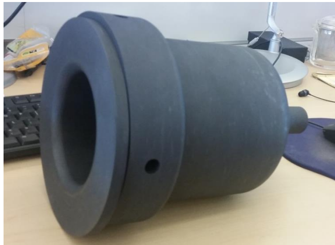
Fig. 32: Experimental laboratory graphite internal receiver. Keyboard in background for size reference.
