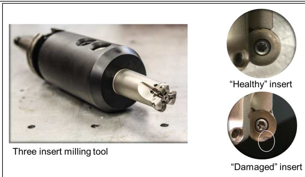
Figure 12: Milling tool and possible insert conditions
