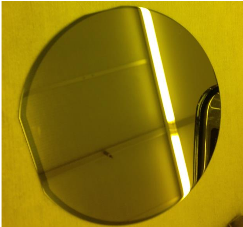
Figure 3.4 NiFe film remains intact e-beam evaporation performed with the chamber heated.
