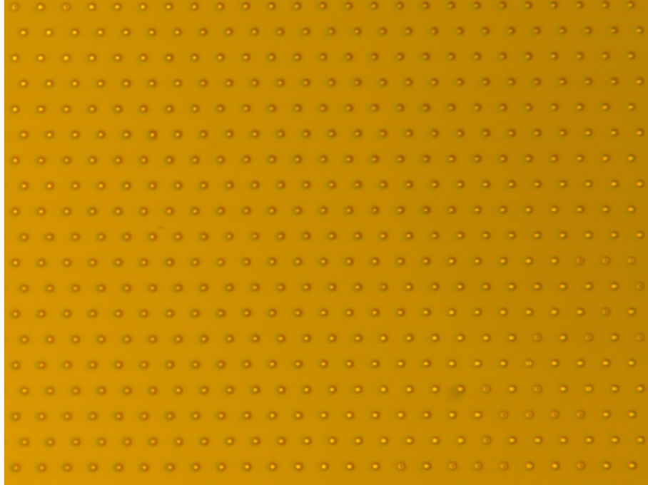
Figure 3.14 Following PECVD SiO 2 deposition, the NiFe features were protected from a piranha etch solution for 10s, indicating the SiO 2 coating is properly protecting the features.
