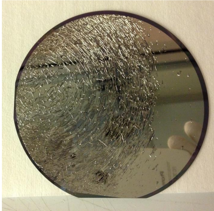
Figure 3.3 NiFe film peeling after deposition. After e-beam evaporation the NiFe film would peel away from the Ti adhesion layer beneath it. This result was seen with various evaporation chamber conditions and substrates.
