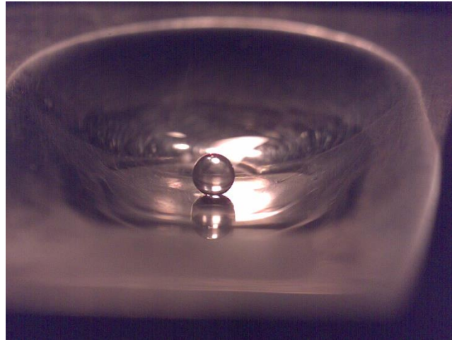
Figure 46 – A single-phase, microliter-volume droplet of silicone oil is levitating, trapped in the bottom of the bowl portion of the polished aluminum substrate. This droplet has a diameter of 1.68 mm.
