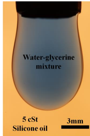
Figure 33 – Image of a pendant droplet of water-glycerine mixture in a 5cSt silicone oil bath used for measuring interfacial tension.
