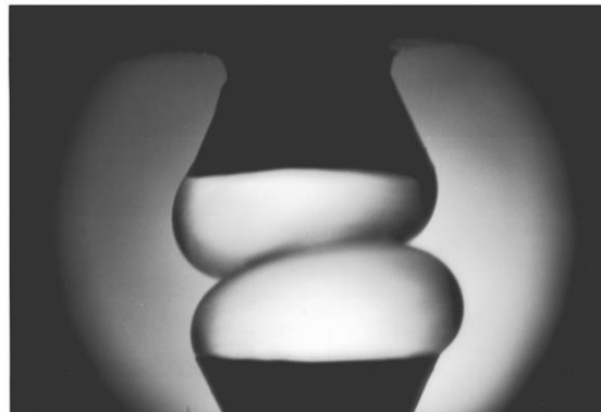
Figure 10 – Permanent noncoalescence via thermocapillary convection between two silicone oil drops pinned at the edges of pedestals (DellAversana et al. 1996).
