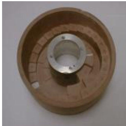
Figure 3.5 Range Modulation Wheel [10]
