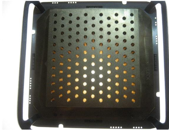
Figure 1.3: Collimator Used for Grid Therapy [2]
