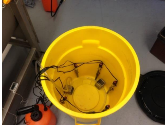
Figure 4.6: 44 gallon trash can converted to a heating apparatus with five 400W Hydor THEO Heaters.
