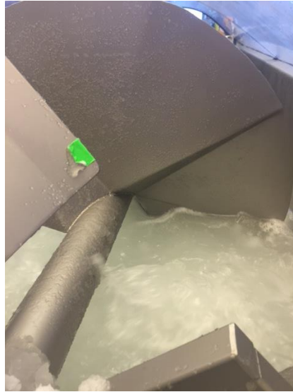
Figure 4.7: 250 gallon auger chiller filled to the center shaft with ice slurry (approximately 125 gallons).
