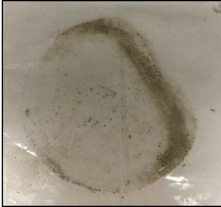
Figure 11: Photo of film after removal showing deposits attached
