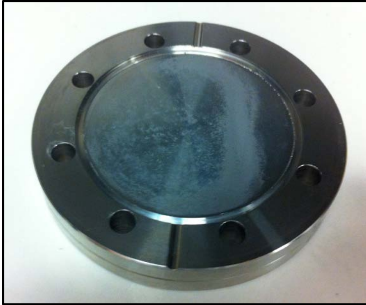
Figure 9: Photo of back side of entry window of target Hg-1, top of assembly is to the left to the photo
