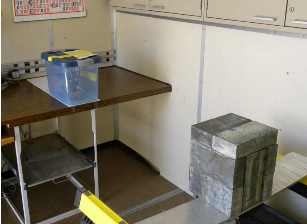
Figure 4: Photo of LANSCE facility HPGe measurement setup, detector-to-target distance was adjusted by moving target towards the back of the table
