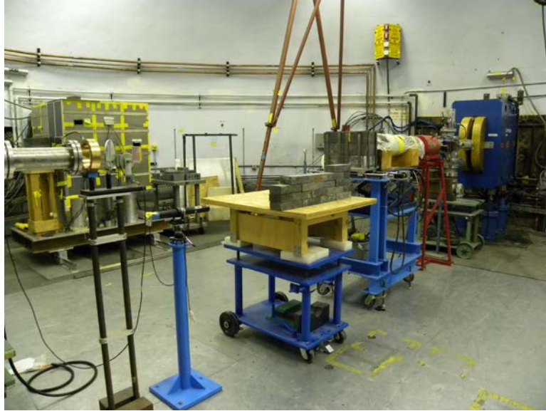
Figure 5: WNR Blue room setup for irradiation of targets. Protons enter from left
