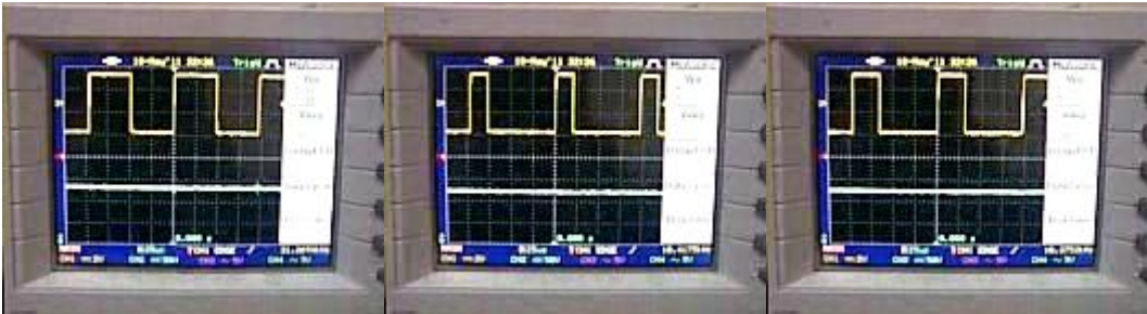
Figure 6-22: Examining the PWM output with close loop controller.
