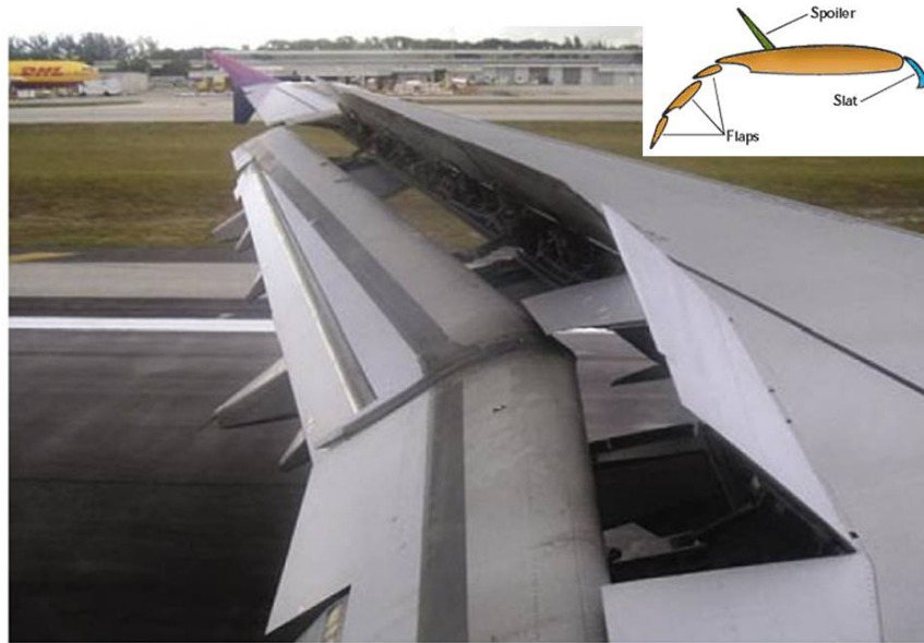
Figure 45: Example of spoiler deployment on aircraft
