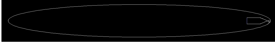
Figure 20: Elliptical cross-section airfoil with jet flap
