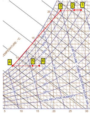
Figure 5.11: Building AHU monitoring schematic Figure 5.12: Air state change conditioned by AHU
