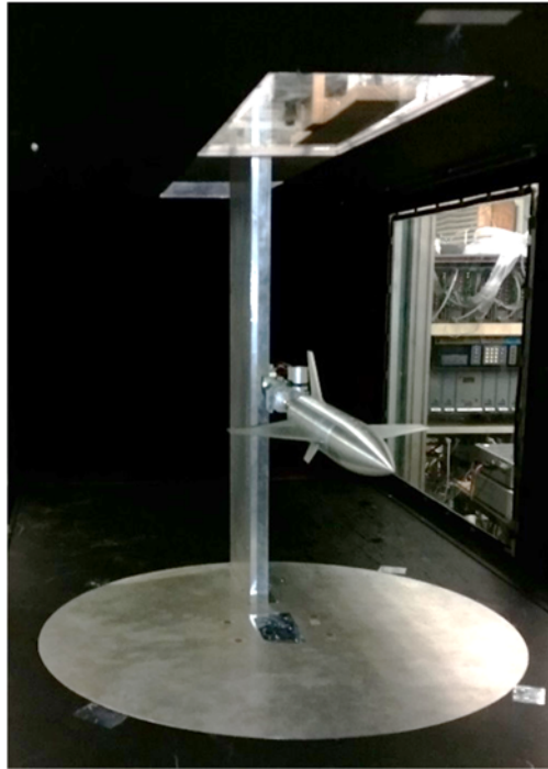
Figure 42 Model Support System Installed in Test Section
