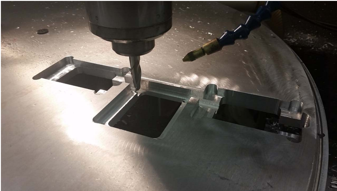
Figure 39 Turntable Replacement during Fabrication
