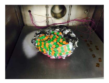
Figure 55. Ruptured Benzoic Acid Test Article Showing White Benzoic Acid Residue
