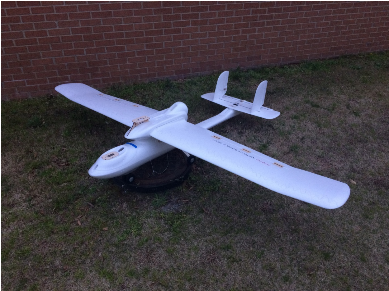
Figure 30: Air Titan FPV Airframe
