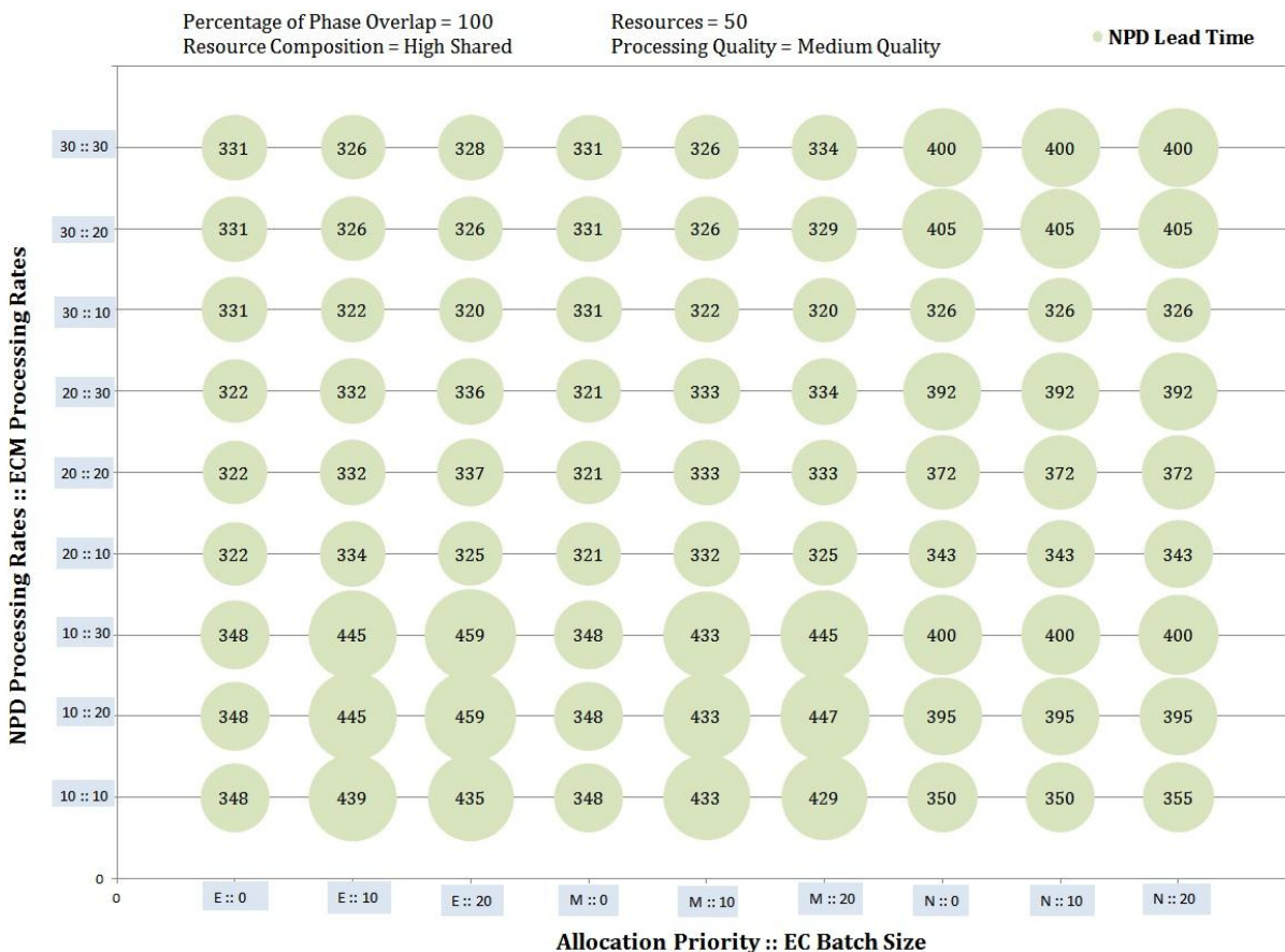
Figure 41: Influence of NPD and ECM processing rates, and allocation priority and EC batch size, on NPD lead time (resources 50)
