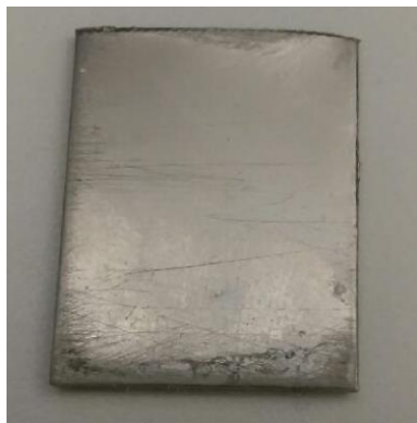
Fig. 50. The Titanium pellet 2cm*2.5cm used as an electrode.
