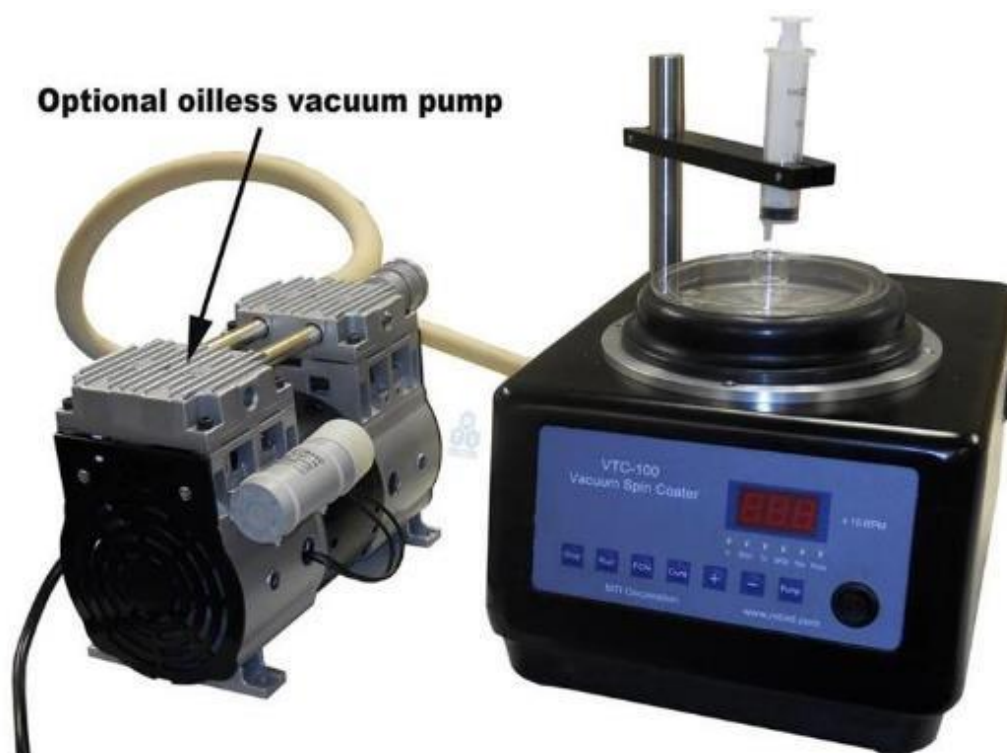
Fig. 53. Spin coater MTI Corp. Model VTC-100.
