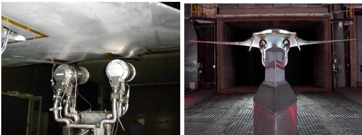
Figure 36 Hybrid Wing Body Model in 14x22' Tunnel with the CJES Units and Model Support
