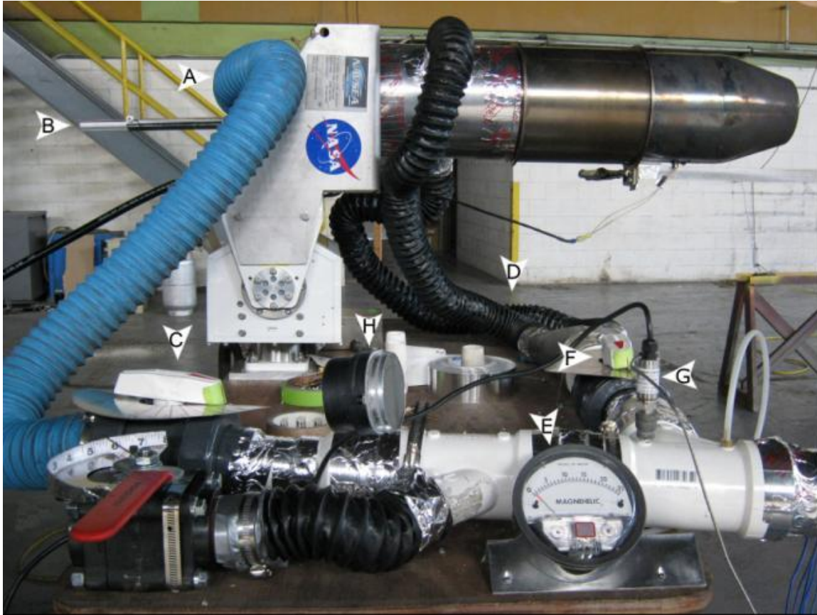
Figure A-3 NAVSEA Jet Engine Simulator- Infrared JES-IR Final Configuration.
