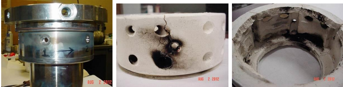
Figure 27 Soot Buildup in the CJES Unit After First Flow Conditioner Run.
