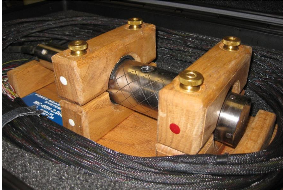
Figure 13: Unitized Multi-Piece Balance
