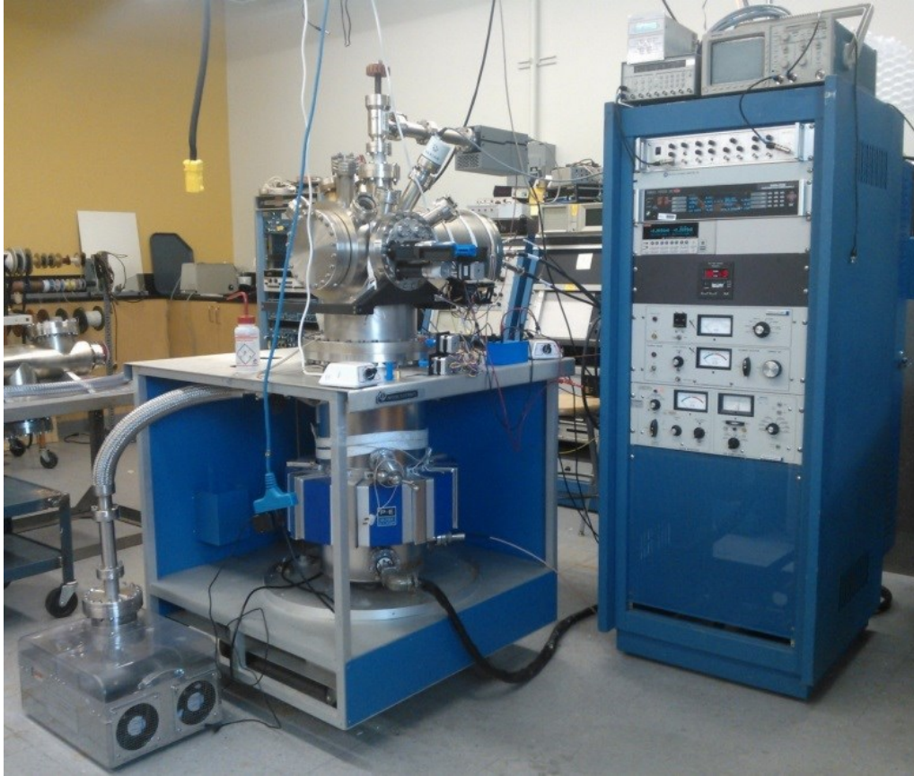
Fig. 4.2 A photograph of the experimental setup for measuring SEY .
