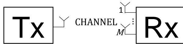
Figure 4: A block diagram of a Receive diversity– SIMO.
