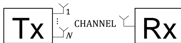
Figure 3: A block diagram of a Transmit diversity– MISO
