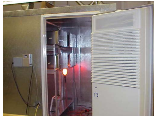
Figure D 2 Small-scale environmental chamber test system
