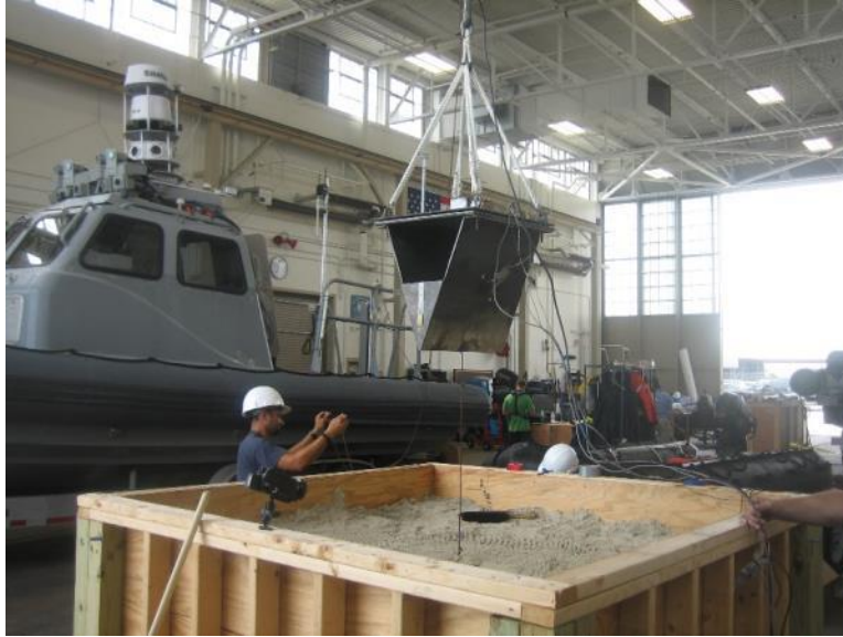
Figure 6. Drop Test Fixture Suspended Above The Sand Box.
