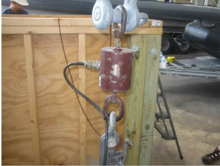
Figure 7. Load Cell and Quick Release Mechanism Used During Testing.
