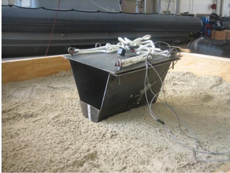
Figure 8. 45° Wedge Fixture Following A Drop Into The Sand Box
