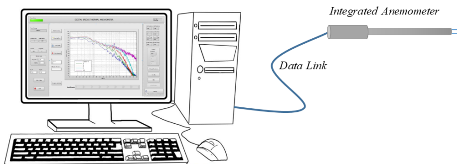
Figure 1.2: DBTA with digital data link
