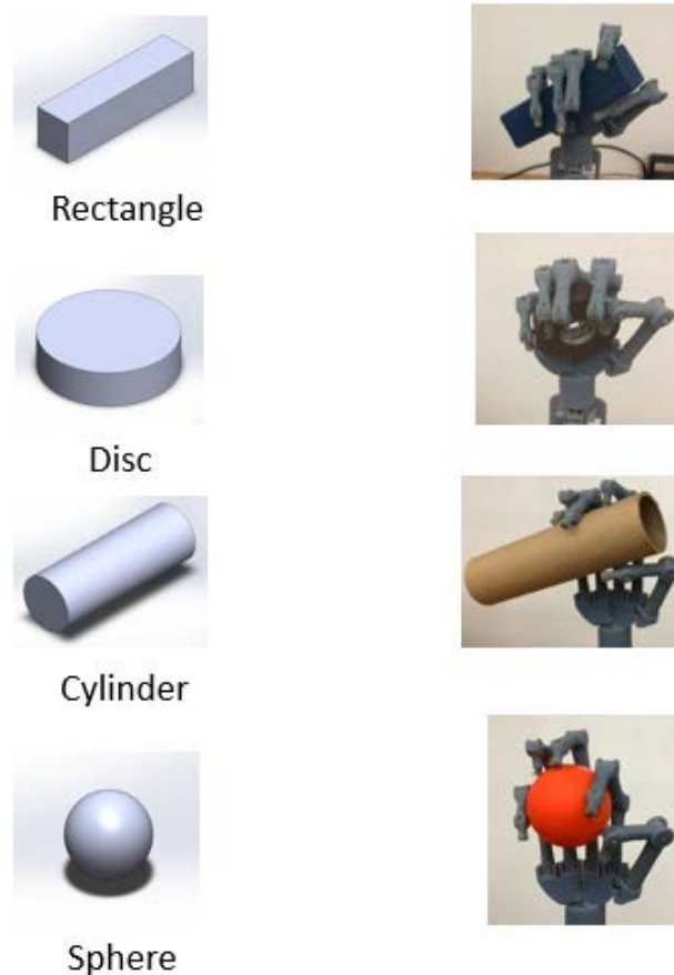
Fig. 5.8. Different grasps performed with hand according to the shapes of objects grasped
