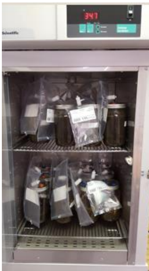
Figure 1 An image showing the general setup used for the anaerobic digestion batch experiments, in which substrate was placed in jars capped with a lids modified to vent into a Tedlar gas sampling bag and placed in an incubator to be maintained at a temperature of 37°C.
