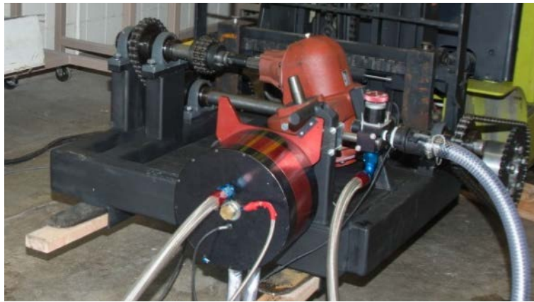
Figure 2.2 Dynamometer (foreground) attached to speed increaser frame and drivetrain to be tested.
