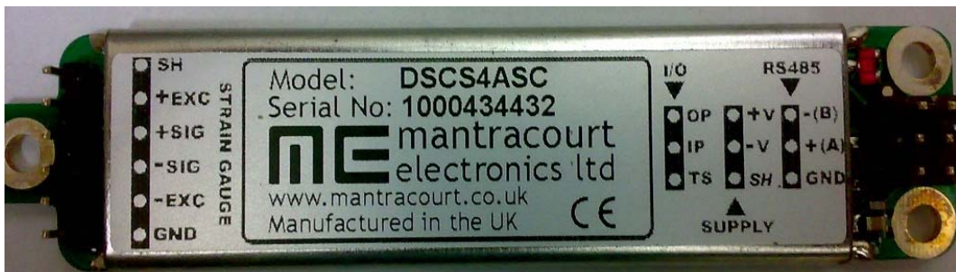
Figure (4.6): The digital strain gage to data converter RS485
