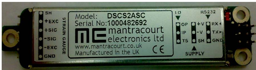
Figure (4.4): The digital strain gauge to data converter with an RS232 output
