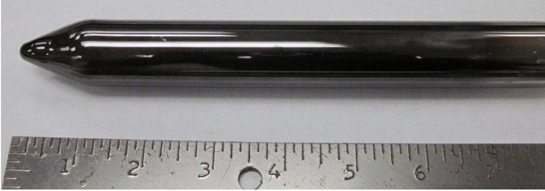
Figure 2.8. Typical quartz ampoule after carbon coating and annealing process is completed.
