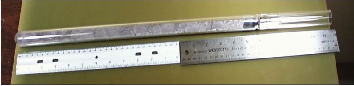
Figure 2.4. Typical zone refined precursor material produced in the laboratory, with impurities segregated to left side of the ampoule, and pure precursor material on right side.
