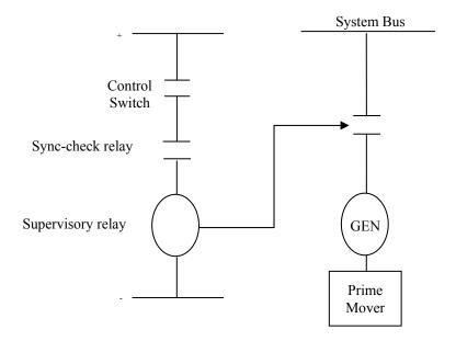
Figure (2.10): Breaker closure with supervisory control
