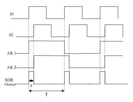
Figure (3.14): Phase angle versus on time of output of XOR gate
