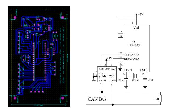
Figure (4.4): Layout of the main PIC 18F4685
