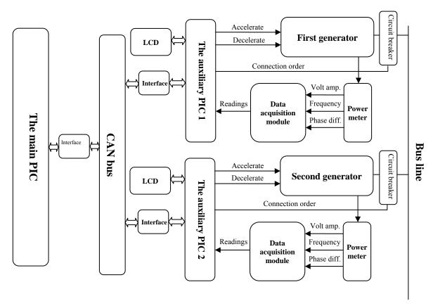
Figure (4.1): The overall system diagram
