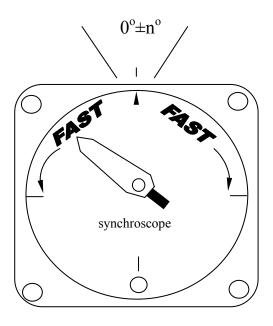
Figure (2.9): Synchroscope
