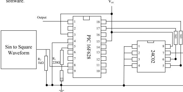
Figure (3.7): Frequency counter circuit
