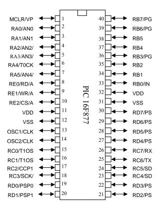
Figure (3.1): Pin diagram of 16F877
