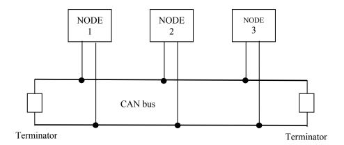
Figure (2.14): Example CAN bus
