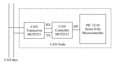
Figure (2.21): CAN node with any PIC microcontroller
