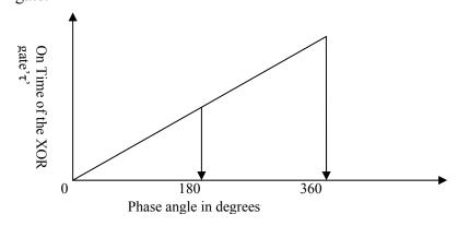
Figure (3.15): Phase angle versus on time of output of XOR gate
