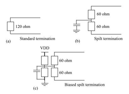
Figure (2.16): Bus termination methods
