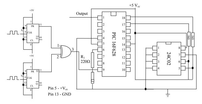
Figure (3.12): Phase meter circuit
