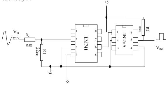
Figure (3.8): Sinusoidal to square waveform converter circuit
