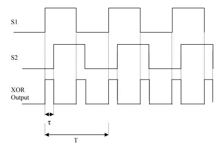
Figure (3.11): Diagram for phase shift
