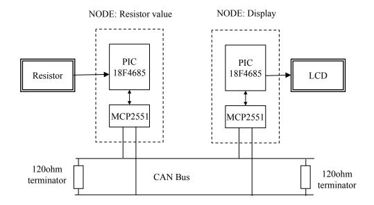
Figure (2.23): CAN block diagram of the example
