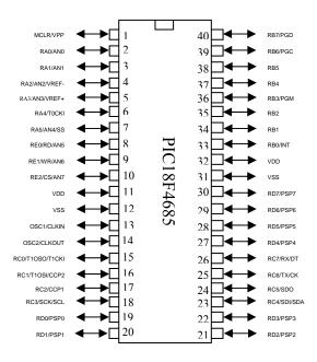
Figure (4.3): Pin diagram of PIC 18F4685
