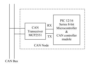
Figure (2.22): CAN node with integrated CAN module
