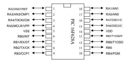
Figure (3.2): Pin diagram of 16F628A
