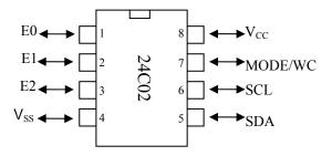
Figure (3.3): Pin diagram of 24C02
