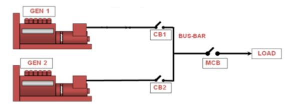
Figure (2.5): Connecting two generators
