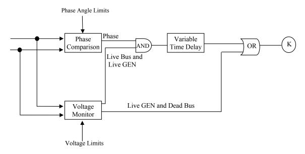
Figure (2.11): Synch-Check block diagram
