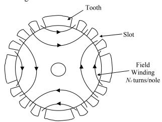
Figure (2.4): A 4-pole cylindrical rotor
