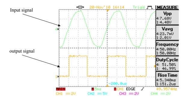
Figure (3.9): The oscilloscope output of the Sinusoidal to square waveform converter circuit
