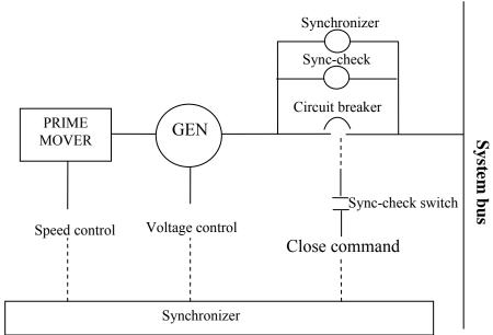
Figure (2.12): Automatic synchronizing
