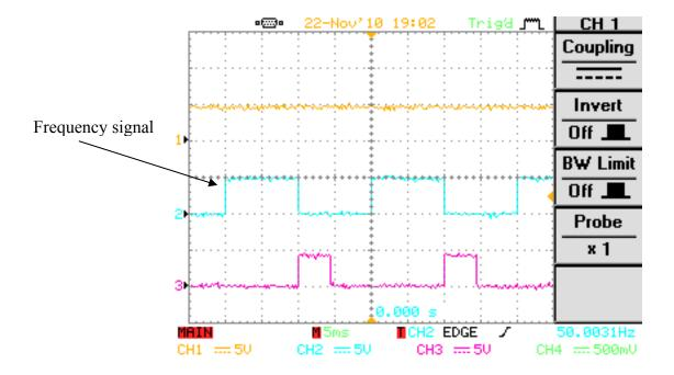
Figure (3.10): The oscilloscope output of frequency counter circuit
