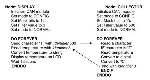
Figure (2.25): Operation of both nodes
