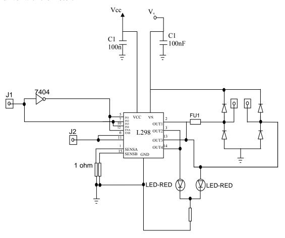
Figure (3.17): Motor driver circuit
