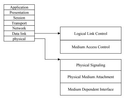
Figure (2.17): CAN and the OSI model
