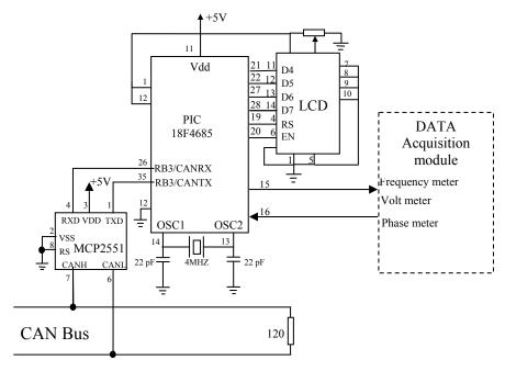
Figure (4.7): The pin connection of the auxiliary PIC with the data acquisition module and LCD
