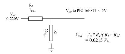
Figure (3.4): Voltage scalar circuit
