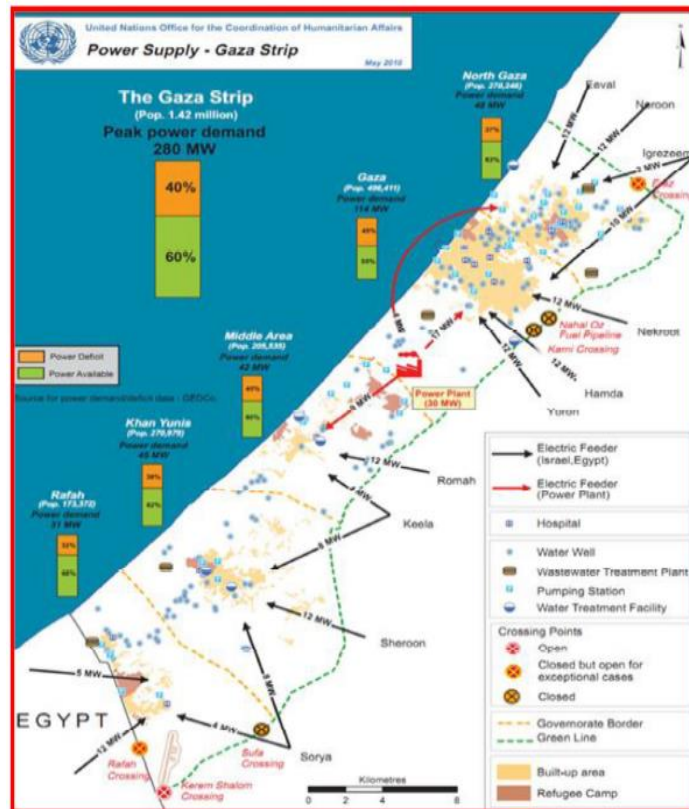
Figure 2.2: Electrical power supply for Gaza Strip in 2010[9]
