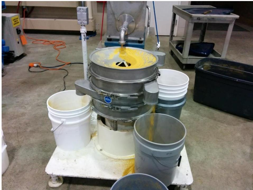
**Figure 3.2.** DDGS sieving using a round sifter Sweco LS18\_333.
