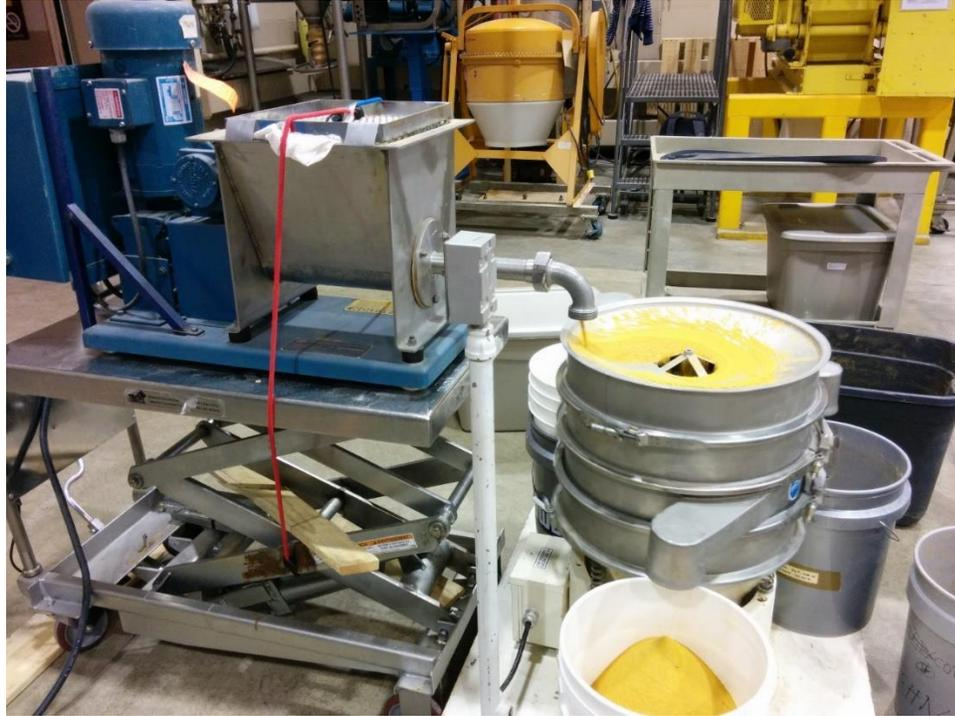
**Figure 3.3.** The process of DDGS sieving.
