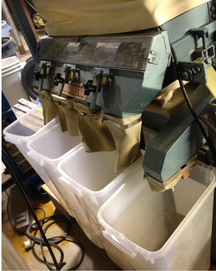
**Figure 3.7.** The collection of four fractions from gravity separation.
