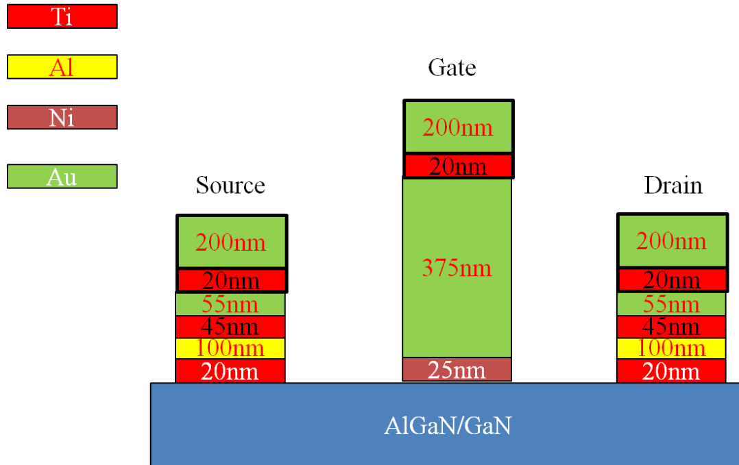
Figure 7.5: Cross section of a HFET embedded AlGaIn/GaN V-shaped microcantilever showing different metal stacks (not drawn to scale).
