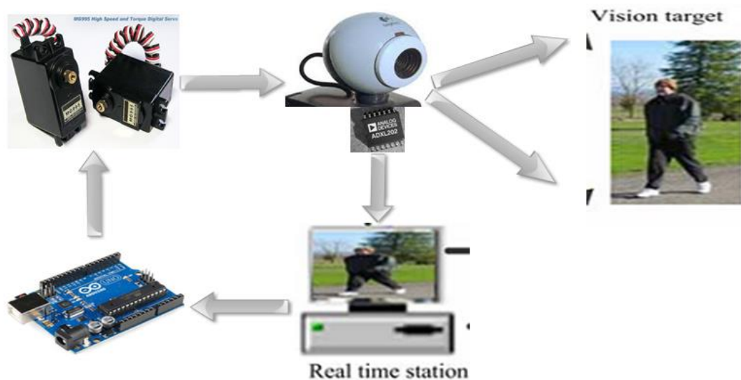
Figure 1.1: Tracking System Components
