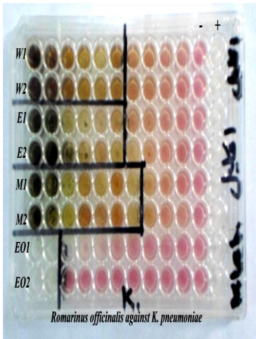
Figure. 4.48. C. W. Aquatic, E. Ethanolic, M. Methanolic & EO. Essintial oil. The MIC & MBC of Rosmarinus officinalis extracts against K. pneumoniae .
